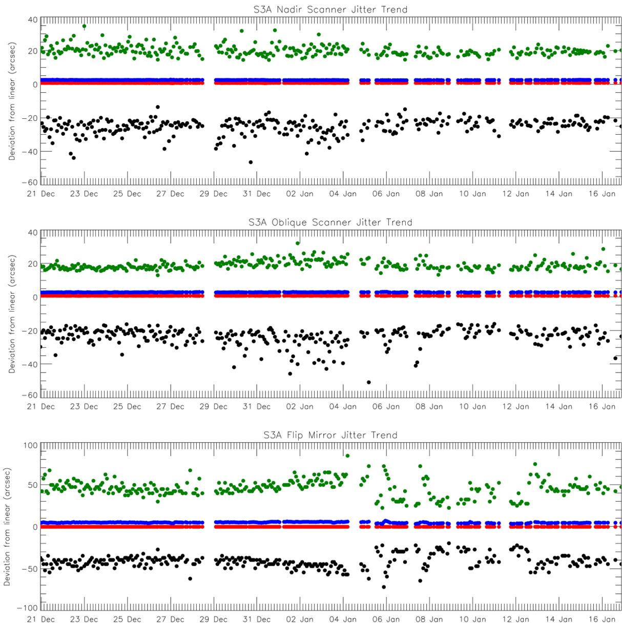
Figure 6: Scanner and flip jitter for cycle 26, showing mean, stddev and max/min position per orbit compared to the expected one for the nadir view.
