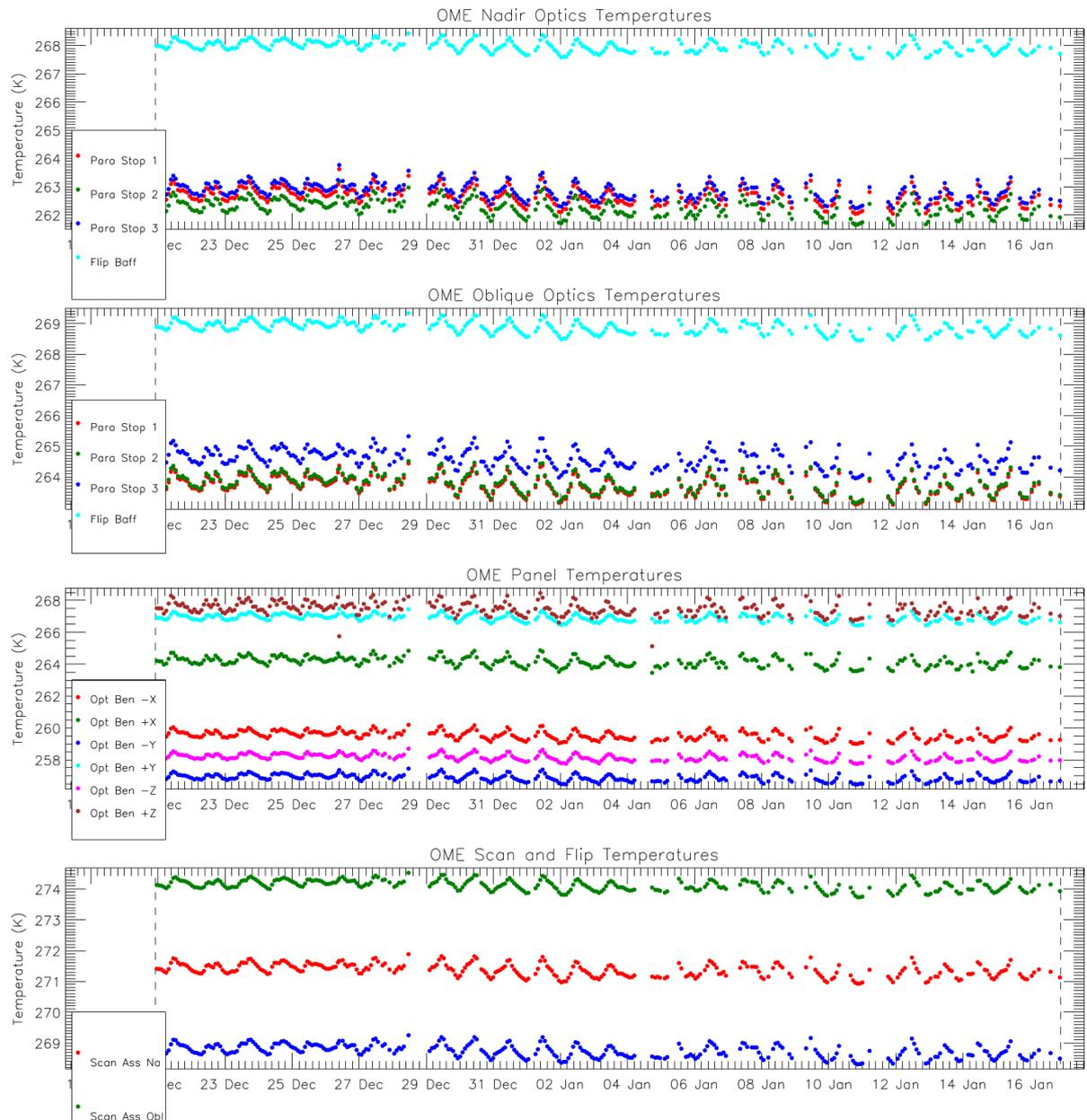
**Figure 5: Opto-Mechanical Enclosure (OME) temperature trends for cycle 26 showing the paraboloid stops and flip baffle (top two plots) and optical bench and scanner and flip assembly (lower two plots). The vertical dashed lines indicate the start and end of the cycle. Each dot represents the average temperature in one orbit.**
