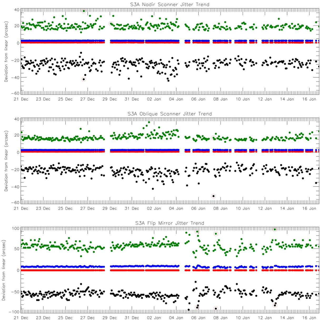
**Figure 7: Scanner and flip jitter for cycle 26, showing mean, stddev and max/min position per orbit compared to the expected one for the oblique view.**
