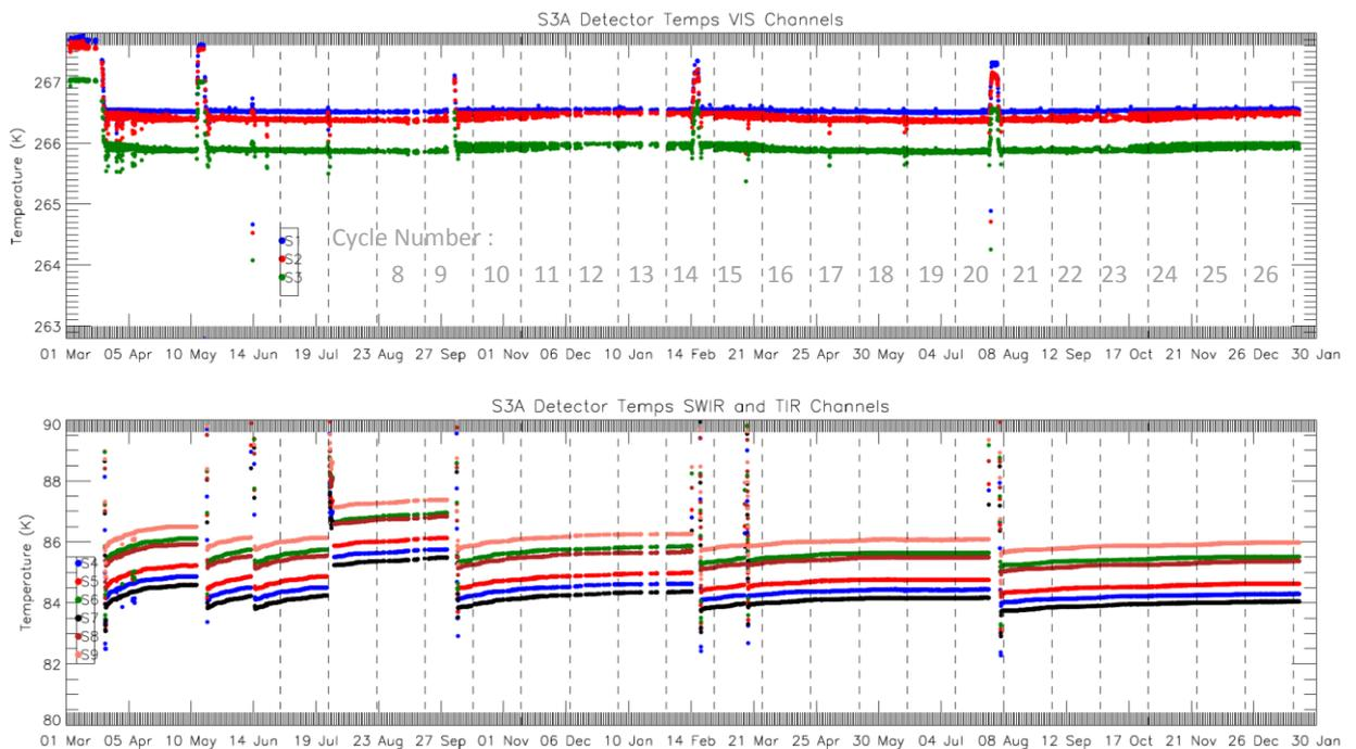
**Figure 1: Detector temperatures for each channel from 1st March 2016. Discontinuities occur for the infrared channels where the FPA was heated for decontamination or following an anomaly. The vertical dashed lines indicate the start and end of each cycle. Each dot represents the average temperature in one orbit.**
