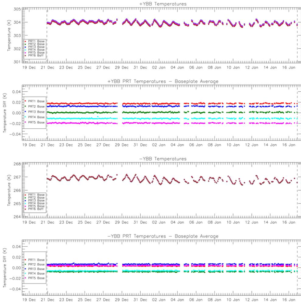
**Figure 2: Blackbody temperature and baseplate gradient trends during cycle 26. The vertical dashed lines indicate the start and end of the cycle. Each dot represents the average temperature in one orbit. Note that the gaps are in the stream of data from the MPC used for monitoring, and are not due to any problem.**
