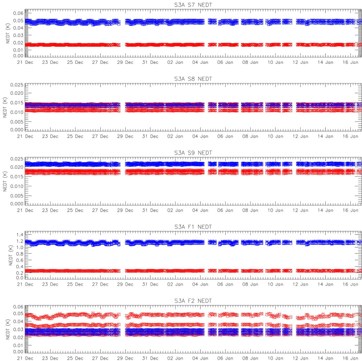
**Figure 9: NEDT trend for the thermal channels in cycle 26. Blue points were calculated from the cold blackbody signal and red points from the hot blackbody. The square symbols show results calculated from the nadir view and crosses show results from the oblique view. Results are plotted for all detectors and integrators, which is why there are several different levels within the same colour points (particularly for S8 and F2).**
