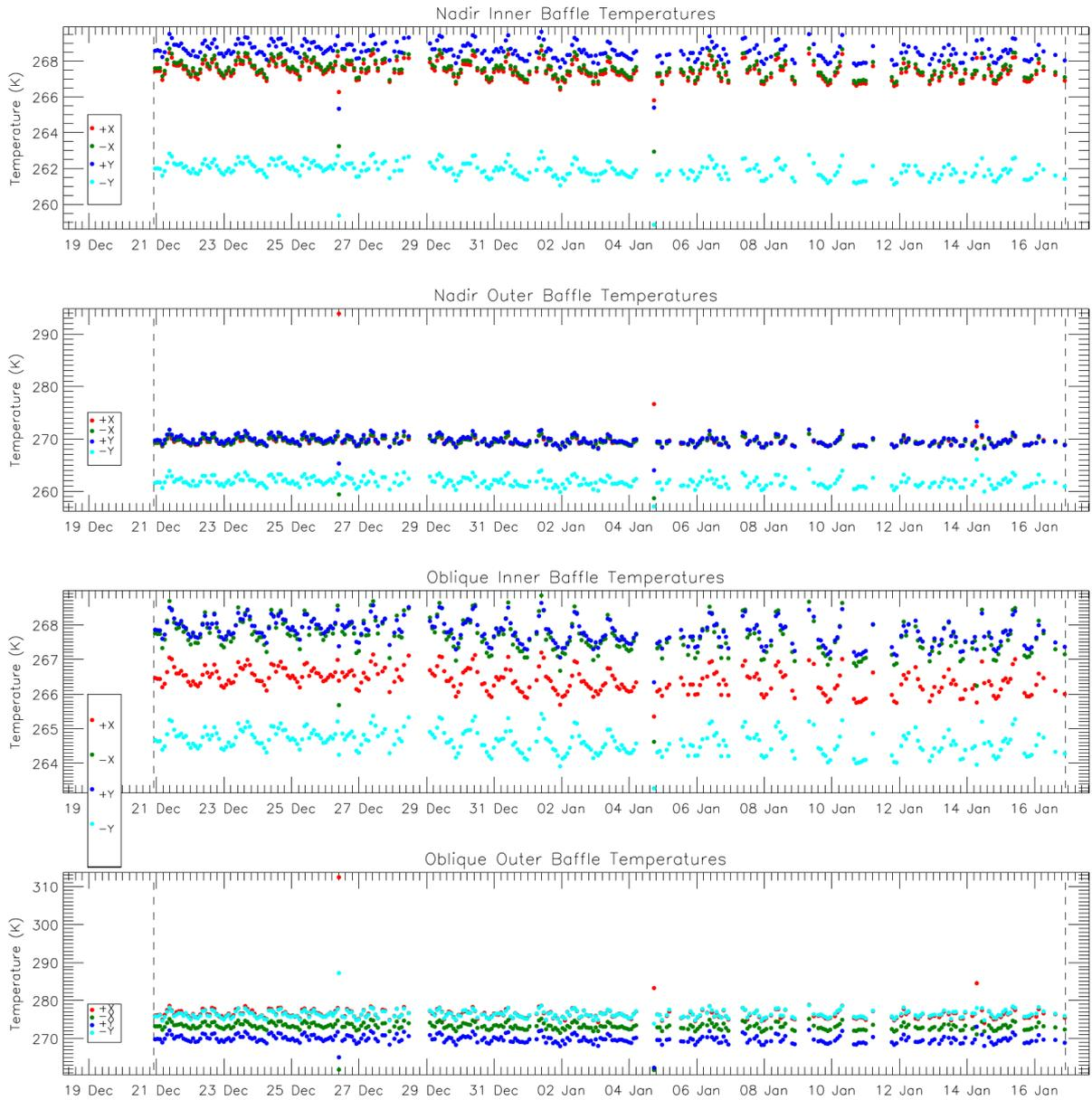
**Figure 4: Baffle temperature trends for cycle 26. The vertical dashed lines indicate the start and end of the cycle. Each dot represents the average temperature in one orbit.**
