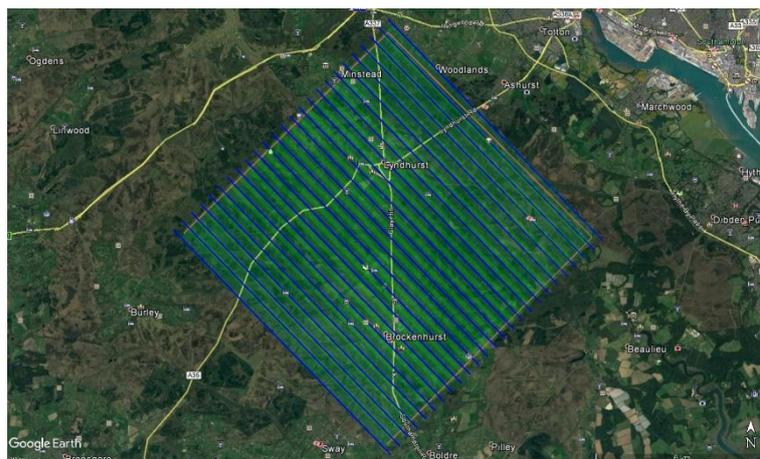
Planned flight lines covering the SP-Val (top) and UK-NFo (bottom) site.
