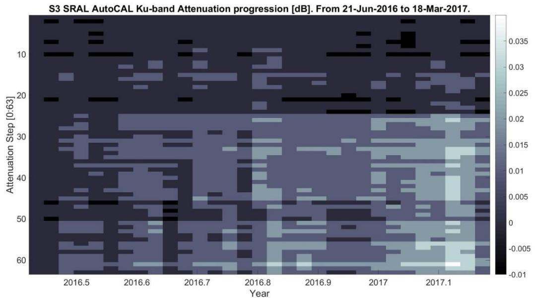
Figure 2.4-11. AutoCAL attenuation whole mission progression for Ku-band. Difference in dB with respect to the previous attenuation value, for each attenuation step.
