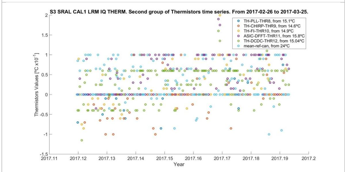
Figure 2.2-36. Second group of Thermistors time series on CAL1 LRM IQ mode. The temperatures are averaged for each calibration product over the analysis period.
