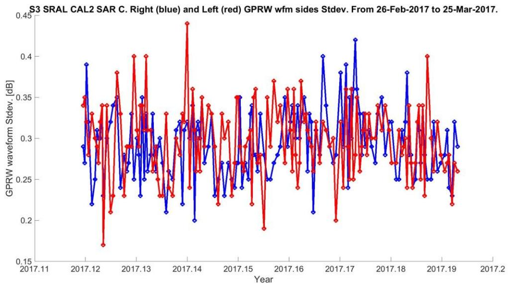
Figure 2.2-32. CAL2 C waveforms right (blue) and left (red) sides Standard Deviation over the period.
