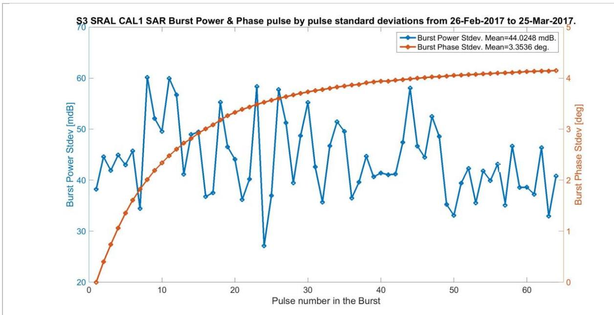
Figure 2.2-24. Pulse by pulse standard deviations of the CAL1 SAR Ku Power and Phase intra-burst corrections.
