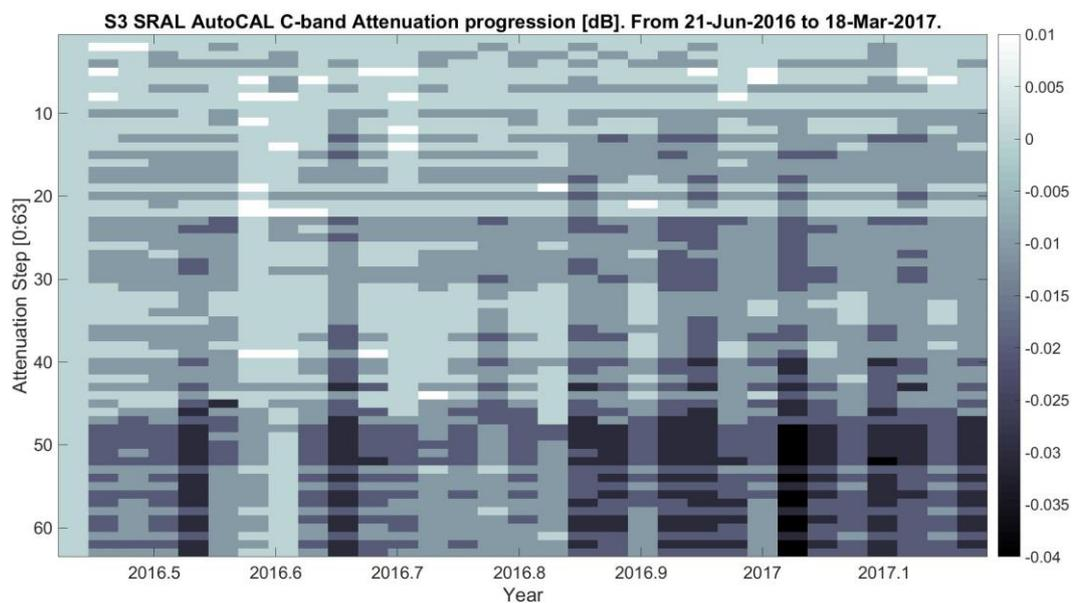
Figure 2.4-12. AutoCAL attenuation whole mission progression for C-band. Difference in dB with respect to the previous attenuation value, for each attenuation step.
