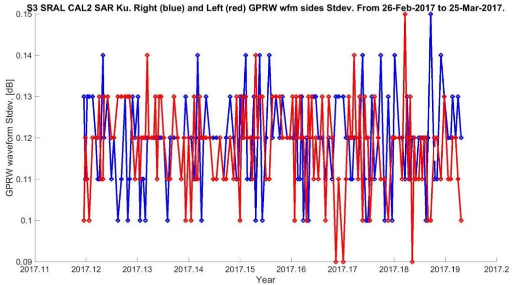
Figure 2.2-31. CAL2 Ku waveforms right (blue) and left (red) sides Standard Deviation over the period.
