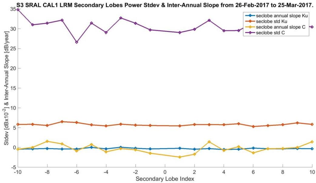
Figure 2.2-10. CAL1 LRM PTR secondary lobes characterisation. The inter-annual slope (in dB/year) and standard deviation (in dBx10<sup>-2</sup>) of each of the secondary lobes during the period are shown.
