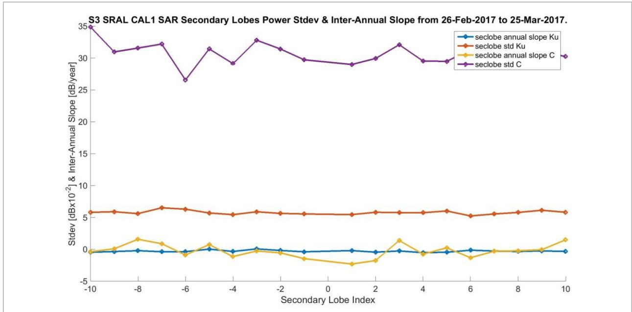
Figure 2.2-20. CAL1 SAR PTR secondary lobes characterisation. The inter-annual slope (in dB/year) and standard deviation (in dBx10<sup>-2</sup>) of each of the secondary lobes during the analysed period are shown.
