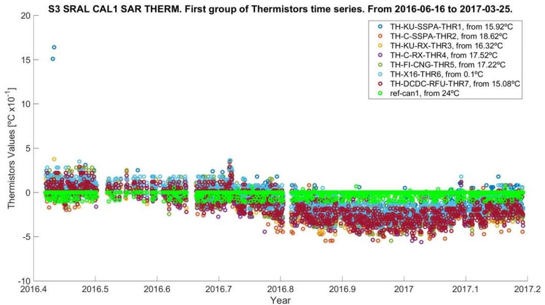
Figure 2.4-13. CAL1 SAR thermistors series along the whole mission. First group.
