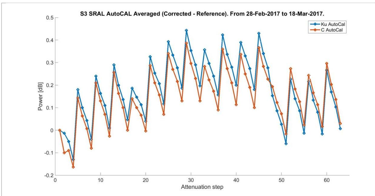
Figure 2.2-34. AutoCal measurements: Corrected - Reference. Averaged over the analysis period.
