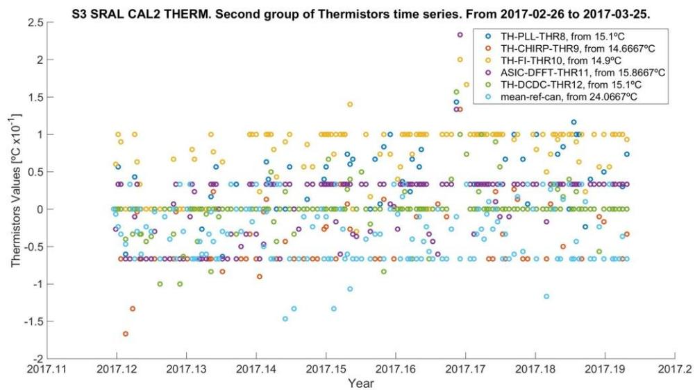
Figure 2.2-40. Second group of Thermistors time series on CAL2 mode. The temperatures are averaged for each calibration product over the analysis period.
