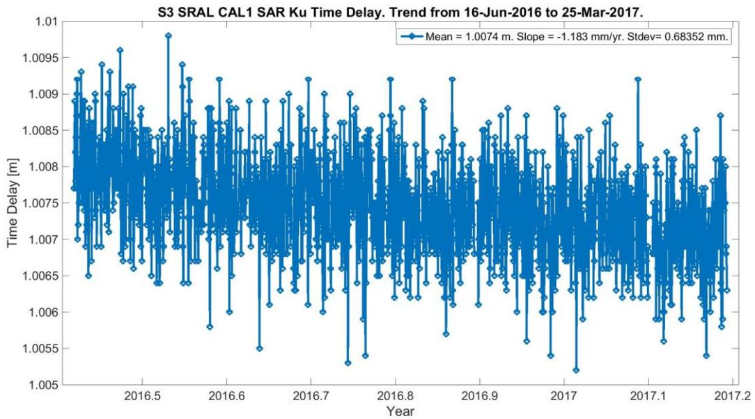
Figure 2.4-1. CAL1 SAR Ku Time Delay Whole Mission Trend.
