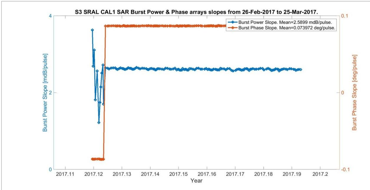
Figure 2.2-23. CAL1 SAR Ku Phase & Power intra-burst corrections slopes over the analysis period.
