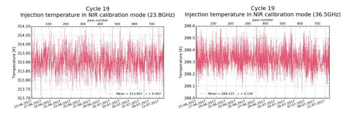
Figure 4: Monitoring of Noise Injection temperature for both channels: 23.8GHz (left) and 36.5GHz (right)
