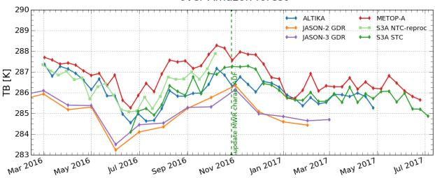
Figure 15 : Average temperature over Amazon forest at 23.8GHz channel for Sentinel-3A, SARAL/AltiKa, Jason2,
