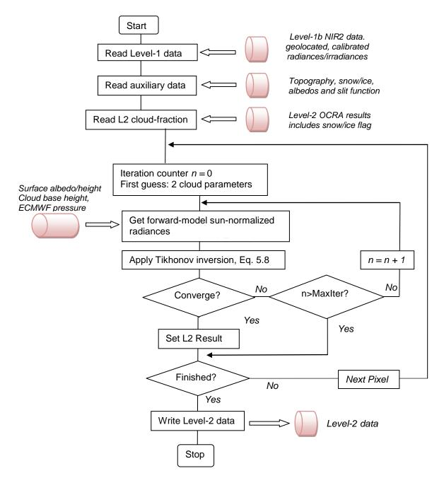
Figure 5.2: Flow Diagram for the S5P\_CLOUD\_ROCINN (CAL) retrieval algorithm.
