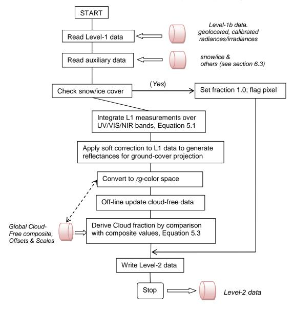
Figure 5.1: Flow Diagram for the S5P\_CLOUD\_OCRA (OCRA) retrieval algorithm.
