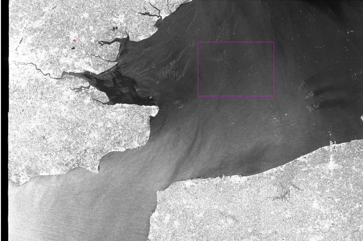
**Figure 69: S-1B IW Image of SE England and N France with the location of range ambiguities indicated (acquisition 5th August 2016, 17:40:17 UT).**
