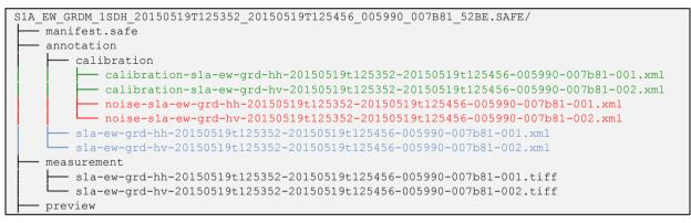
Figure 9: Representation of the product folder tree, with in red the NADS, in blue the LADS and in green the CADS
