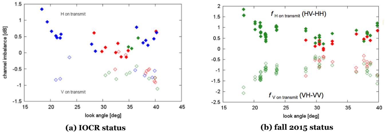
**Figure 1: Channel imbalance between cross- and co-polar channel derived from the transponder IRF for H- (filled diamonds) and V-polarization (open diamonds) on transmit for different modes (blue: SM, red: IW, green: EW).**
