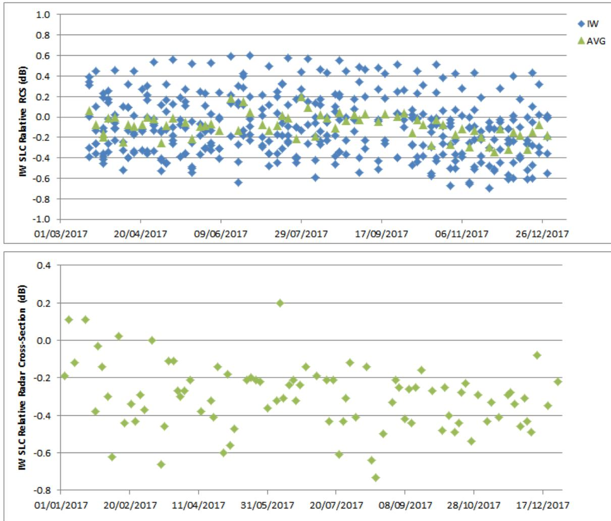
Figure 16: IW SLC Relative Radar Cross-Section for the DLR Transponders and the BAE Corner Reflector
