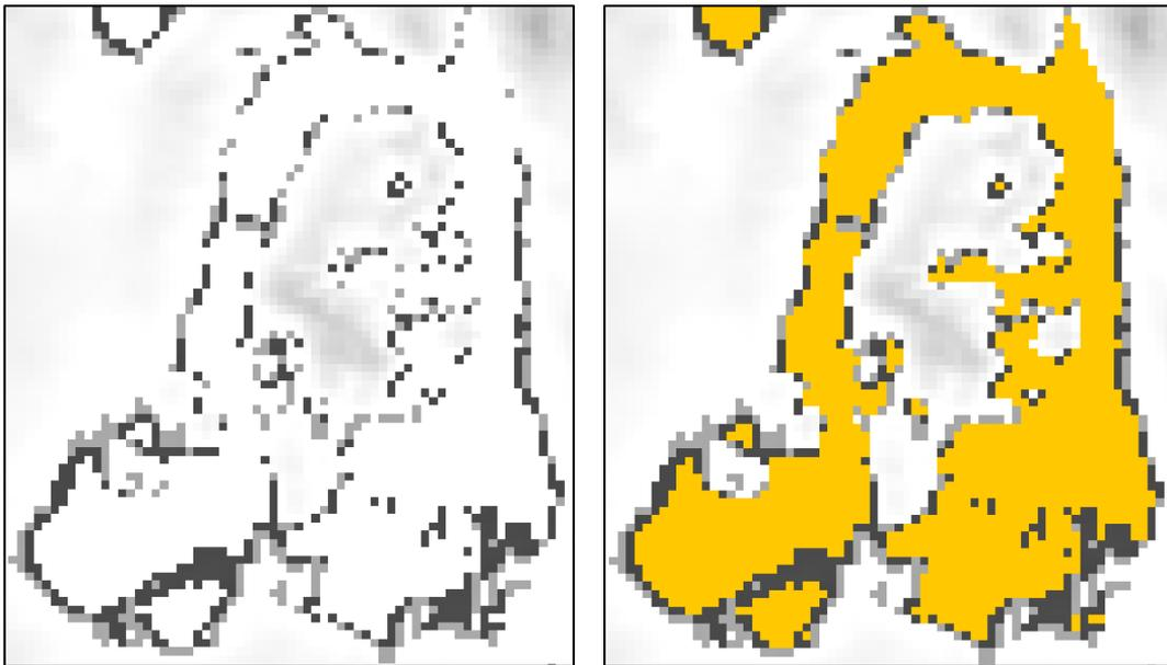
**Figure 1: OLCI-A level 1 radiance for band Oa16. Left: without saturated mask. Right: with saturated mask in orange. Dark and grey pixels form a pattern of low radiance anomalous pixels that do not represent the geophysical scenario.**
