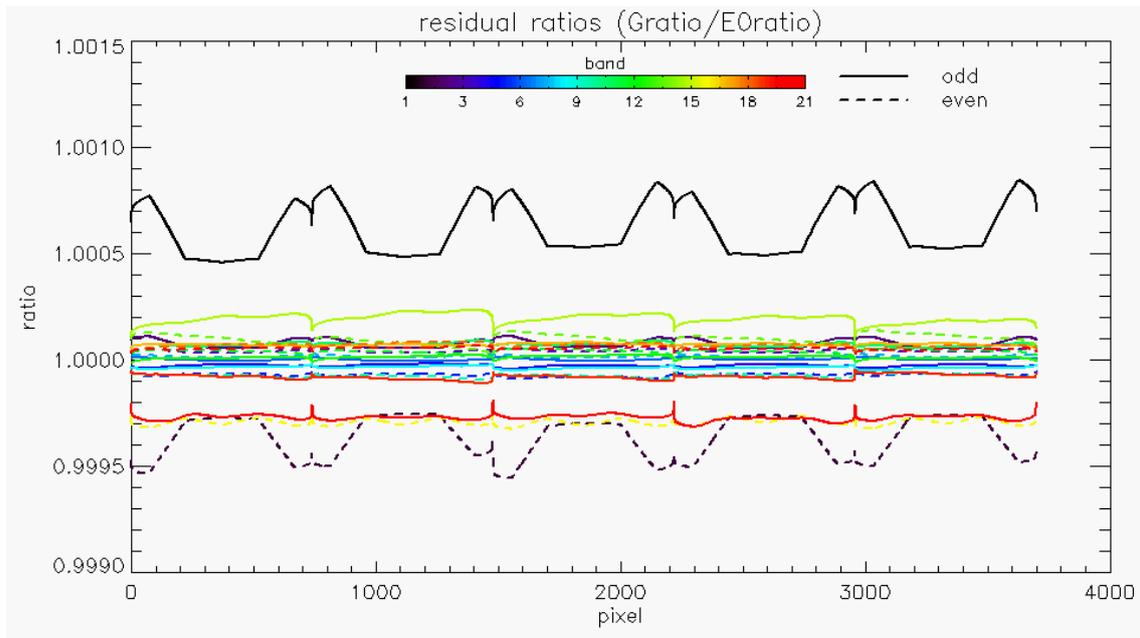
**Figure 29: non-linear residuals introduced by the straylight in the radiometric gain computation.**
