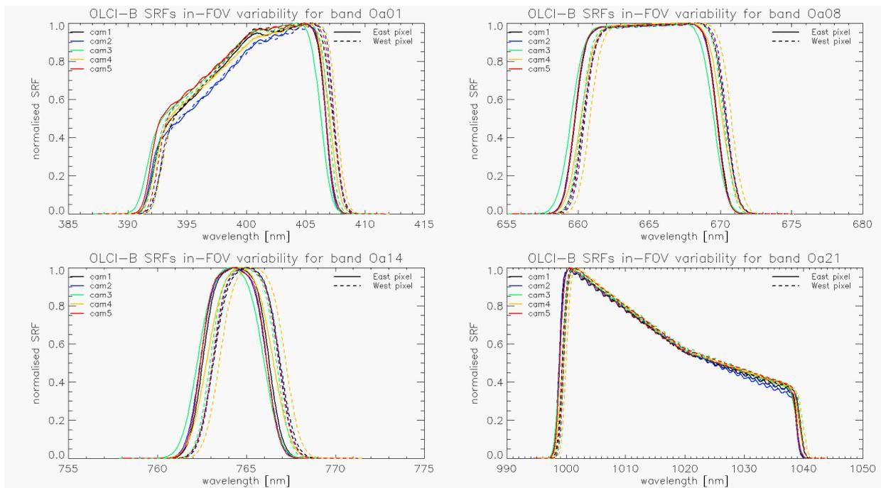
**Figure 4: OLCI-B SRFs in-FOV variability for bands Oa01 (top left), Oa08 (top right), Oa14 (bottom left) and Oa21 (bottom right). SRFs are plotted for each camera (black to red colour) and for two pixels close to the camera edges (solid or dashed line).**
